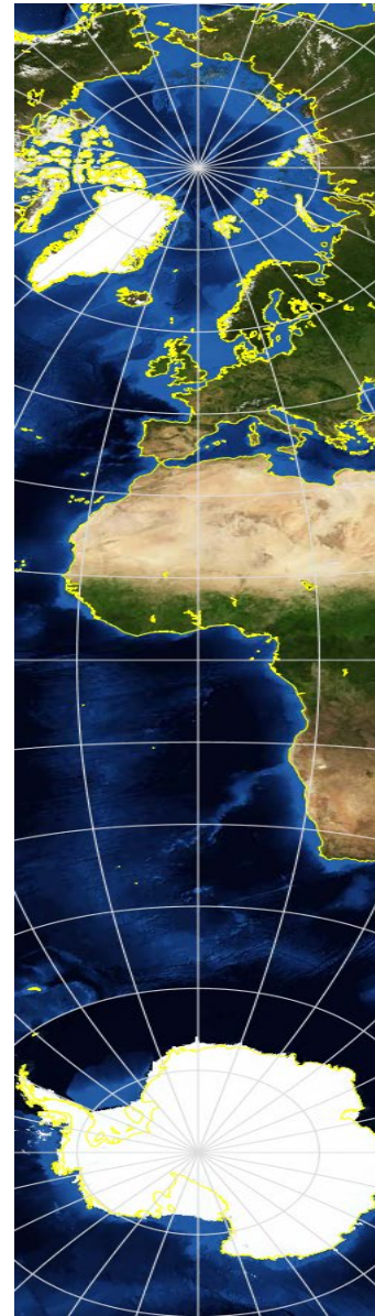
Figure 2 SOCEA Projection for an orbit track along the Prime Meridian. Cropped from:
