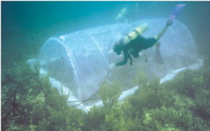
Fig. 4. The Submersible Habitat for Analyzing Reef Quality (SHARQ), a large benthic incubation chamber that allows the 24 h monitoring of water chemistry variations driven by substrate carbon and carbonate metabolic processes
