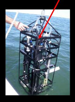
absorption  $a(\lambda)$  attenuation  $c(\lambda)$  backscattering  $b_b(\lambda)$  temperature pressure conductivity
