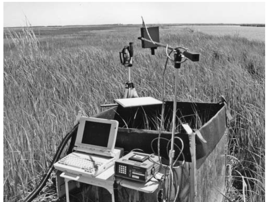
Marsh inundation experiment apparatus (Kearney, Stutzer, Turpie, Stevenson, 2009)
