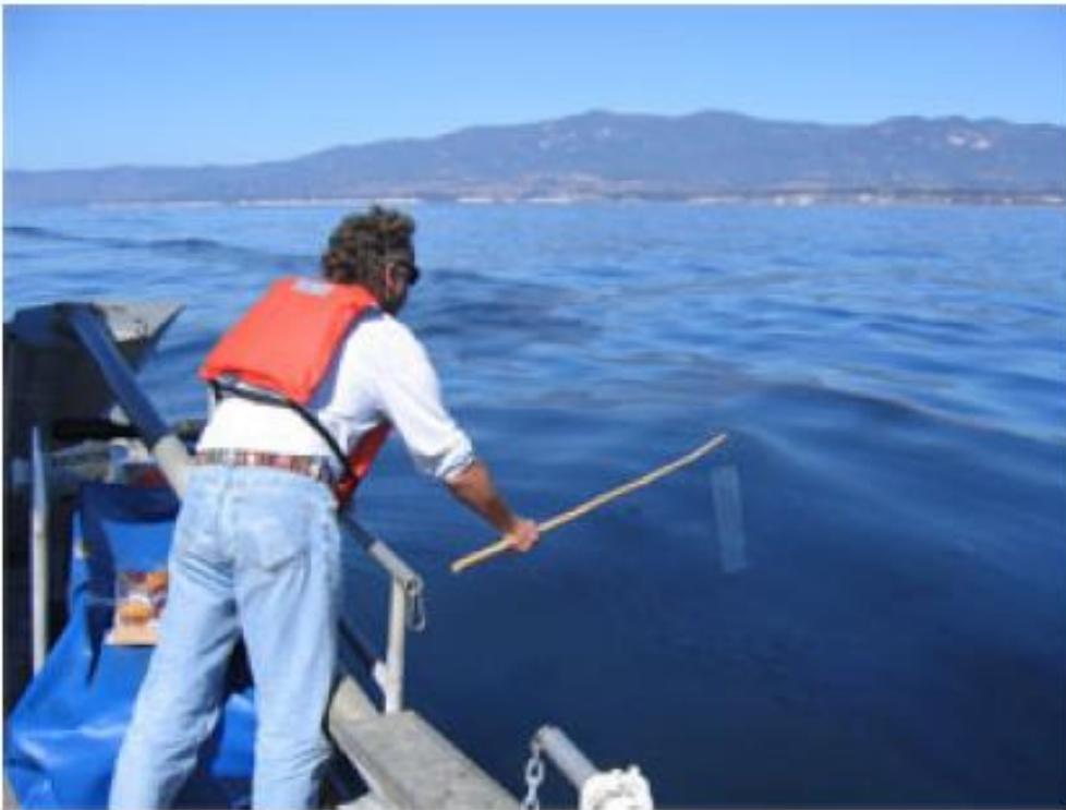
Figure 5. The oil thickness sampling plate being lowered into a Santa Barbara Channel oil slick (left); The same plate after being raised from the slick (right).
