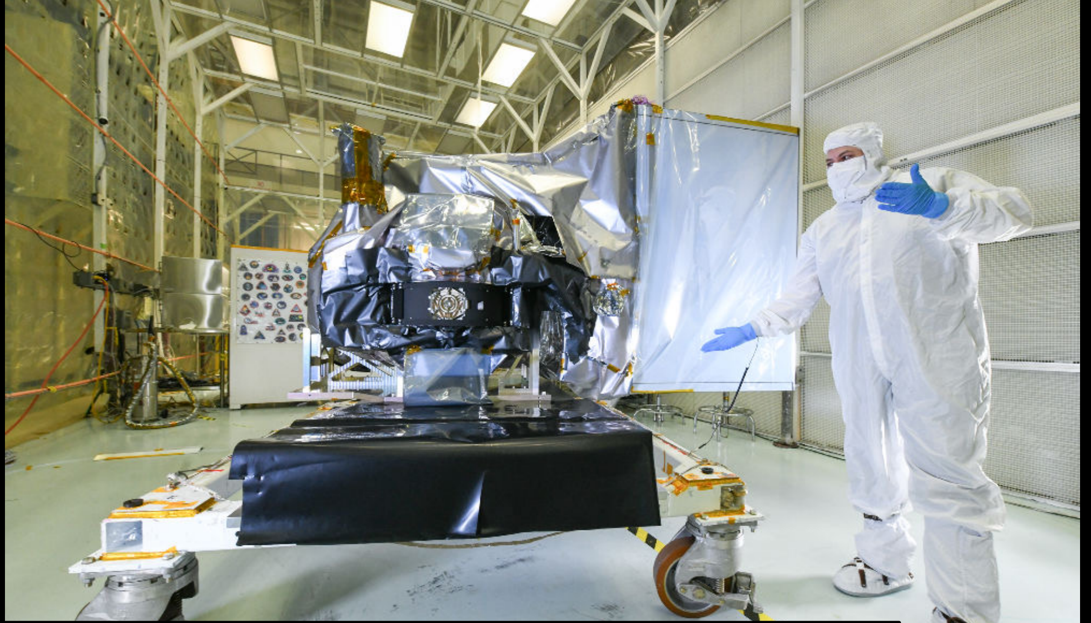
OCI entered thermal vacuum in Aug 2022, where it will remain through Oct 2022 It was successfully mated with the tilt system & passed all structural / mechanical / EMI tests
