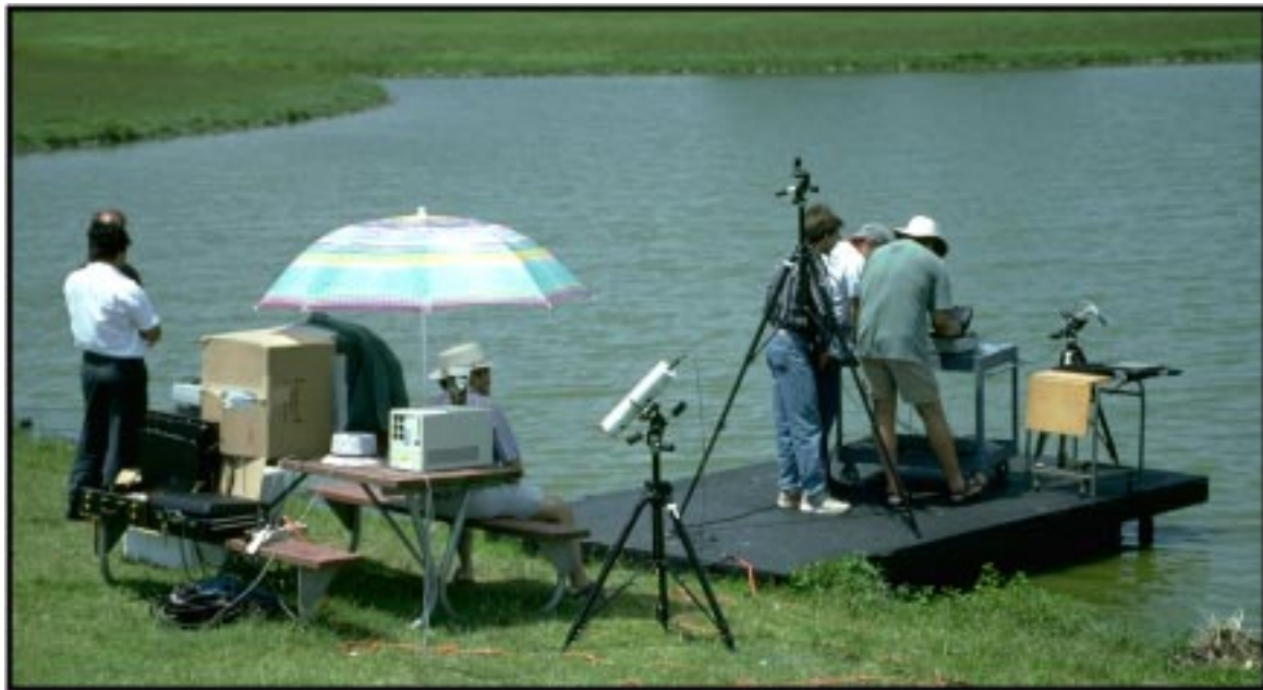
Fig. 5. Photograph of Lab III, illustrating the construction of the experimental platform (black plywood) over the overflow drain, the gray plaque, the SAR and SAI sensors, the GAR sensor, the data acquisition equipment, and some of the participants.
