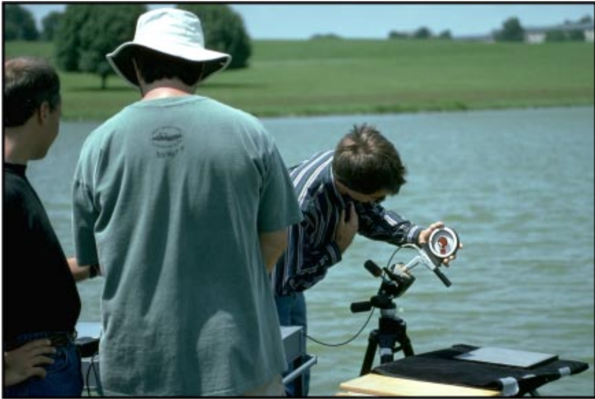
Fig. 6. Photograph during Lab III, illustrating the method used to align the radiance sensors (SAR in this case) to the diffuse plaque. For measurements of L_{\text{sfc}} , the tripod with the sensor was moved to the edge of the experimental platform.
