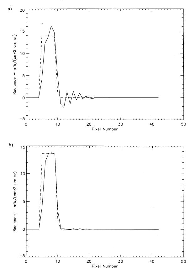
Fig. 12. Ringing from the lunar calibration model for a) high amplitude ringing, b) low amplitude ringing. Note: the dashed line is the target and the solid line is the response.
