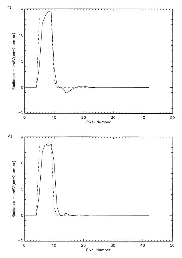
Fig. 12. (cont.) Ringing from the lunar calibration model for c) high frequency ringing, and d) low frequency ringing.
