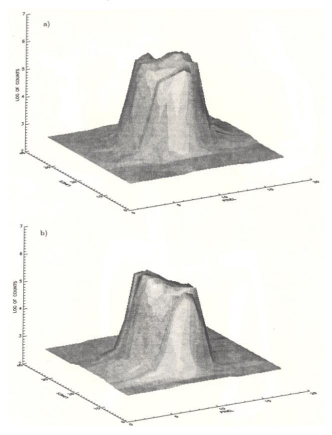
Fig. 19. A three-dimensional representation of a) the lunar sweep at 1922 PST for channel 6 and b) the same scene from the opposite perspective ( $180^{\circ}$  difference).
