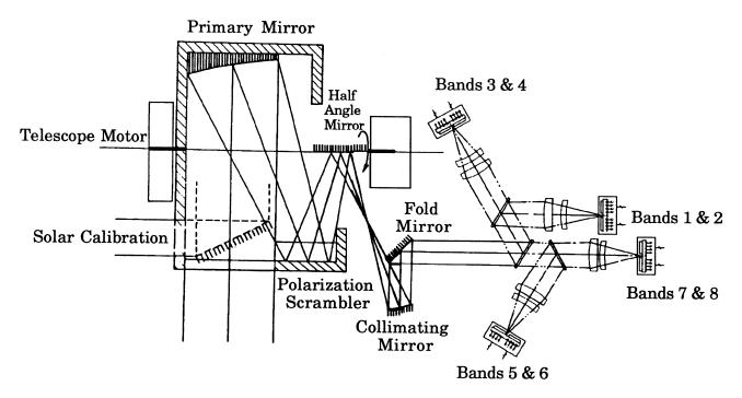
Fig. 17. A schematic of the SeaWiFS optical layout.
