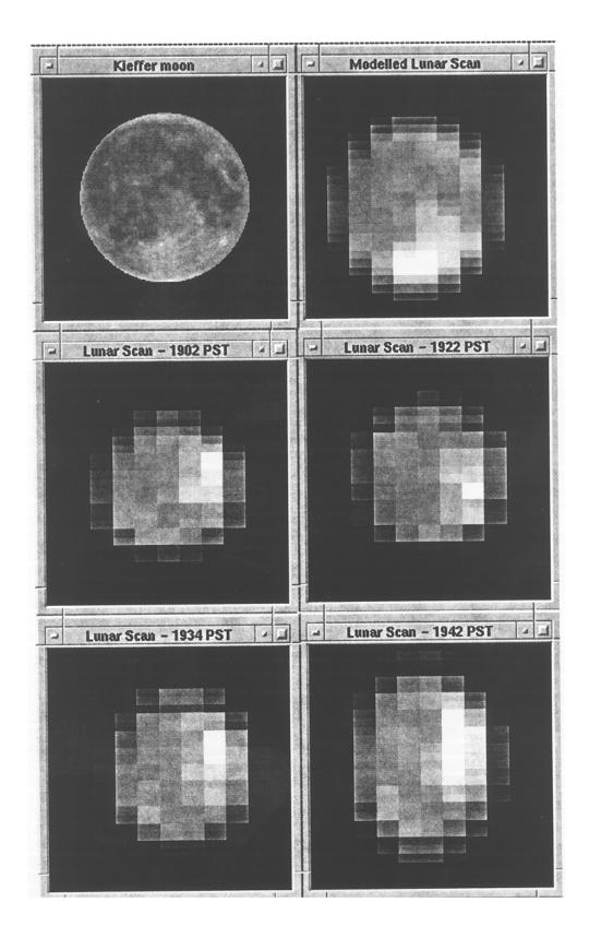
Fig. 16. Comparison of modeled lunar scan to ground-based measurements.
