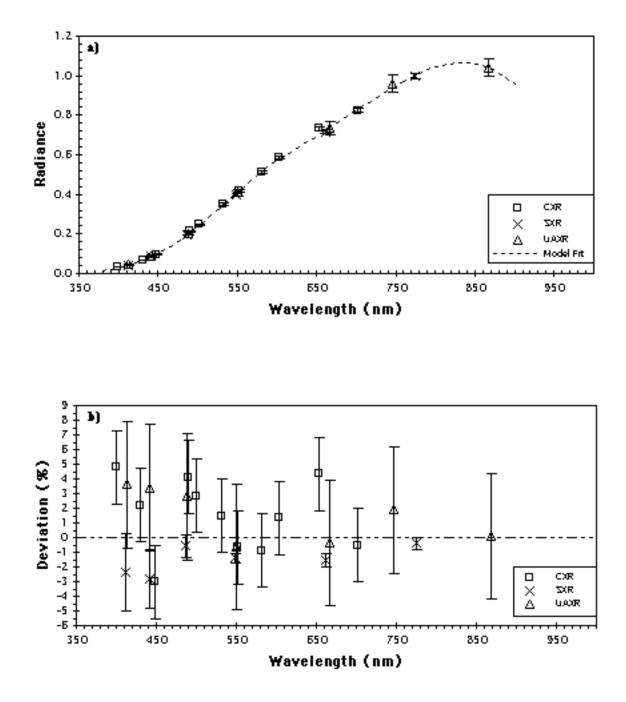
Fig. 19. a) Average spectral radiance in units of  $\mu W/(cm^2 \operatorname{sr} nm)$  of the BSI sphere as measured with the SXR, the UAXR, and the CXR, shown with the model fit to these data. b) Results from panel **a** with respect to the model fit and the uncertainties, calculated as described in the text. The quantity plotted (see legend) is the CXR, SXR, or UAXR data minus the model fit, normalized to the model fit.
