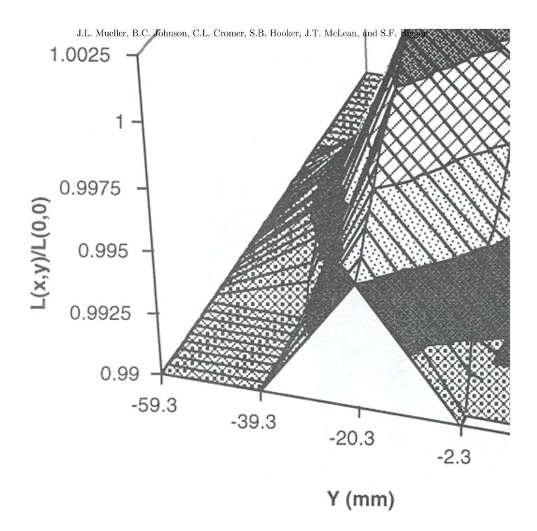
Fig. 28. Spatial variability of the spectral radiance L(531.9), viewed normal to the plane of the exit aperture of the CHORS sphere, as measured with the CXR on 12 and 13 Sept 1994, just prior to SIRREX-3. The values are plotted relative to the radiance measured at the center of the exit aperture, i.e., at (x, y) = (0 mm, 0 mm).
