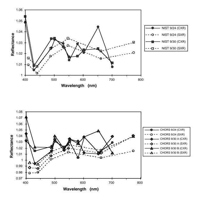
**Fig. 34.** Reflectance factors of the NIST (panel **a**) and the CHORS (panel **b**) plaque using the SXR (dashed lines and open symbols) and the CXR (solid lines and filled symbols) at a viewing angle of 45°. The plaques were illuminated with H91534 (SIRREX-3 data) at a distance of 150 cm. The CHORS plaque was cleaned between the A and B measurements on 30 Sept 1994.
