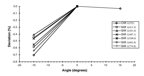
Fig. 31. Lambertian quality (angular uniformity of radiance) of the CHORS sphere, measured within  $15^{\circ}$  of the normal to the center of the plane of the exit aperture using the SXR (all wavelengths) and the CXR (531.9 nm only). The quantity plotted is the spectral radiance at a particular viewing angle minus the spectral radiance at normal incidence, normalized to the normal incidence value, for the indicated measurement wavelengths of the SXR and the CXR.
