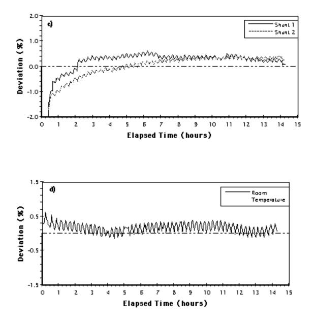
Fig. 24. (cont.) c) Temporal stability of the voltage measured across the two shunt resistors for the CHORS sphere during the 29–30 September tests, again plotted as deviations with respect to the average. d) Temporal stability of the room temperature during the 29–30 September tests of the CHORS sphere, again shown as deviations with respect to the mean temperature. A few outliers in panels c and d have been replaced with the average of temporally-adjacent data.
