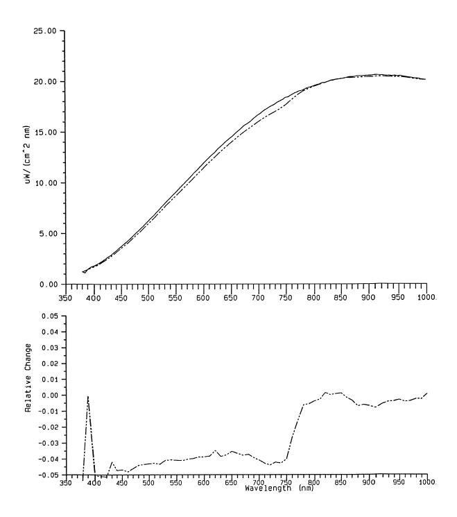
**Fig. 14.** Spectral irradiance of FEL lamp GS-922 determined using F268 on 21 Sept 1994 (solid line), compared to the original calibration by EG&G (dashed line). The spectral irradiance is plotted in the upper panel. The lower panel illustrates the relative changes with respect to the SIRREX-3 values. The quantity plotted using the dash-dot-dot line is the original calibration by EG&G minus the SIRREX-3 data, normalized to the SIRREX-3 data.
