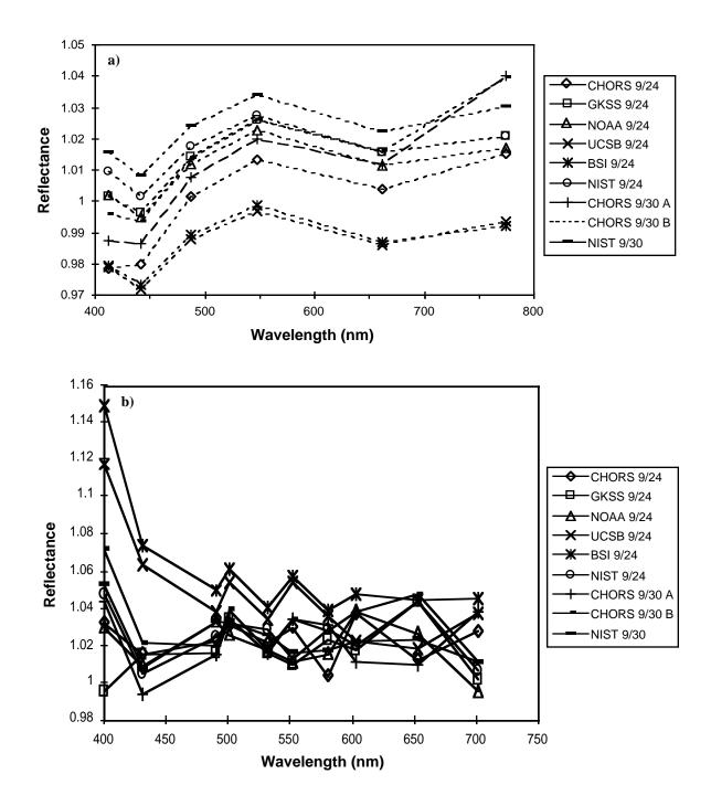
**Fig. 33.** Reflectance factors of all Spectralon plaques (Table A-1) estimated from radiance measurements by the SXR (panel **a**) and the CXR (panel **b**) at a viewing angle of 45°. The plaques were illuminated with FEL lamp H91534 at normal incidence at a distance of 150 cm (148 cm for the UCSB and the BSI plaques). The SIRREX-3 values for spectral irradiance for H91534 (Table 6) was used to calculate the irradiance at the surface of the plaque.
