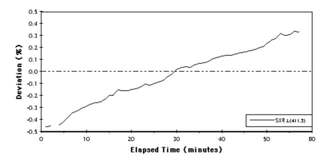
Fig. 25. Temporal stability of the spectral radiance of the BSI sphere as measured with the SXR on 26 Sept 1994, shown as the spectral radiance at 411.5 nm minus the average spectral radiance at this wavelength over the measurement interval, normalized to the average value.
