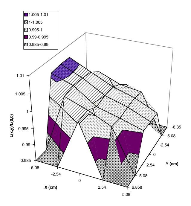
Fig. 29. Spatial variability of the spectral radiance L(487.1), viewed normal to the plane of the exit aperture of the UCSB sphere, as measured with the SXR during SIRREX-3. The values are plotted relative to the radiance measured at the center of the exit aperture, i.e., at (x, y) = (0 cm, 0 cm). Note that unlike Figs. 27 and 28, the x and y axes have been plotted here in reverse orientation.
