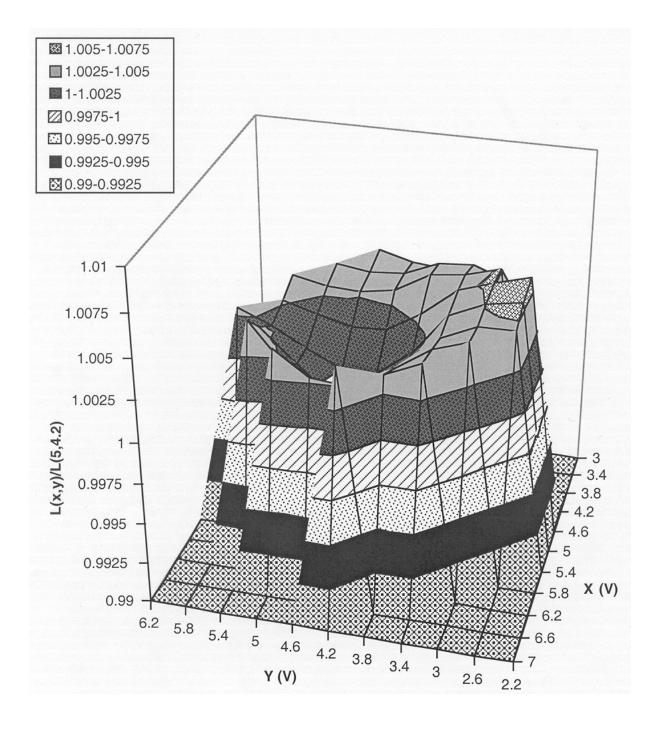
Fig. 27. Spatial variability of the spectral radiance L(487.1) viewed normal to the plane of the exit aperture of the GSFC sphere, as measured with the SXR on 9 Sept 1994. The values are plotted relative to the radiance at the center of the exit aperture, i.e., at (x, y) = (5.0 V, 4.2 V). Variability of similar shapes and amplitudes was measured at 411.5 nm and 774.8 nm.
