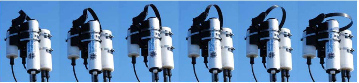
Fig. 53. A sequential movement of the shadowband over the C-OPS solar reference (center white cylinder) on a clear-sky day. The shadowband controller is the right-most cylinder, and the GPS is the left-most. The solar reference is slightly above the other two devices to ensure an unobstructed view of the sky. The primary cable connection is to the controller; the other devices plug into the controller to receive power and send data. The black cylinder between the BioGPS and the solar reference is a solar reference for another instrument system.
