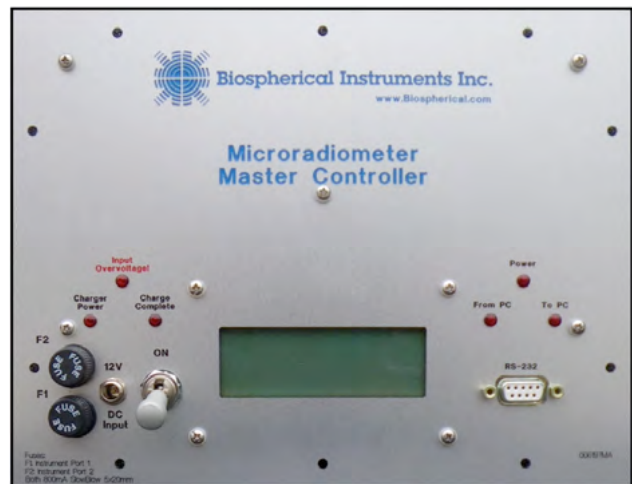
Fig. 37. The front panel of the deck box used with optical instruments built with the MMS architecture. The LCD is the green rectangle in the bottom-middle portion of the panel.
