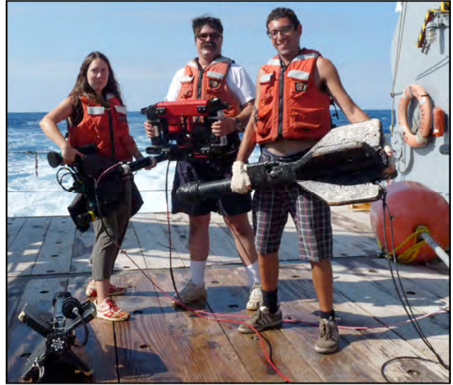
Fig. 49. Three generations of AOP profilers, which were deployed during one of the Bermuda Atlantic Time Series (BATS) cruises in 2009 (left to right, respectively): Natasha McDonald holding a Micro-Pro, which was based on the microNESS instrument; Stanford Hooker holding the first C-OPS unit; and Vincenzo Vellucci holding an SPMR. A second SPMR is on deck in the foreground at left.
