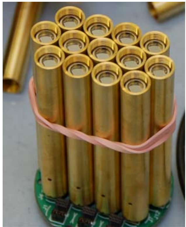
Fig. 28. Completed microradiometers are individually sleeved in brass and may be assembled in arrays on an aggregator board. Shown are 13 individual microradiometers.
