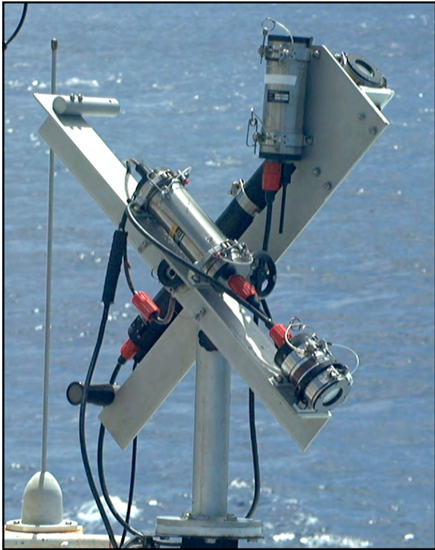
Fig. 1. The SeaSAS frame with the rails oriented at approximately 40^\circ with respect to nadir and zenith. The pointing module is attached to the upper right rail (vertically orientated).
