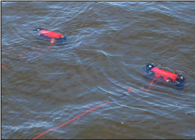
Fig. 45. The C-OPS (left) and SuBOPS profilers (right) deployed simultaneously for operational evaluation. The two instrument systems are shown in a river system with a water depth of approximately 6 m.
