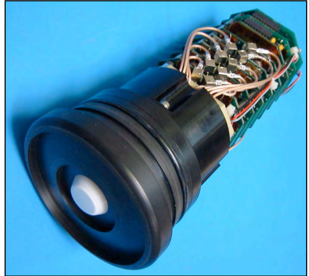
Fig. 40. A PRR-800 irradiance sensor with pressure housing removed. Visible are individual coaxial cables conducting the detector photocurrents to a stack of five input amplifier boards (with four channels per board). Completing the stack is an ancillary input board for temperature, pressure, and angle, the microprocessor board, and the multiplexer digitization board.
