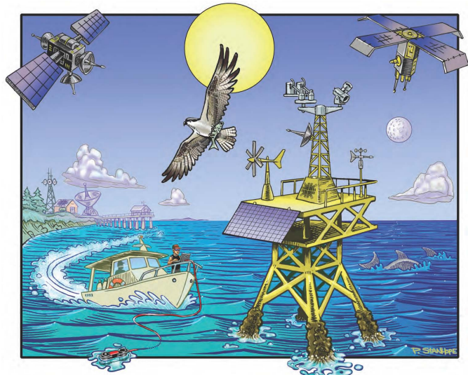
Fig. 3. An OSPREy system showing two sensor sets on top of an offshore tower measuring the atmosphere and ocean, an ocean color satellite sampling the on- to off-shore (green to blue) productivity gradient, the Sun and Moon as calibration targets, a communications satellite for data (including meteorological) telemetry, solar panels and a wind generator for power, a shore-based support facility, and a small boat for monthly validation—including next-generation in-water AOP profiles—and maintenance visits.
