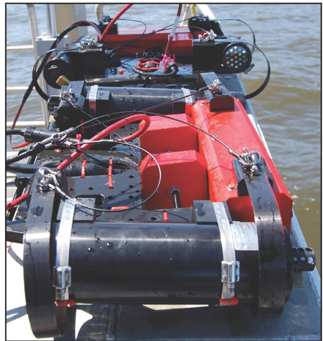
Fig. 20. The SuBOPS instrumentation with the extra T probe fitted inside a perforated shroud for protection and mounted on the L_u sensor end cap (bottom right). The multicolored radiance aperture for C-OPS (Chap. 4) is visible in the background (top right).
