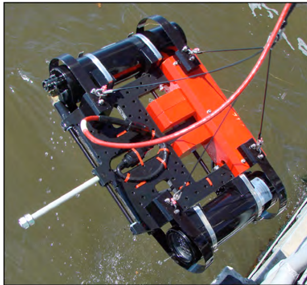
Fig. 18. The SuBOPS instrumentation with the custom-blended foam, which can be machined and shaped (the weighted spar is shown not wrapped in black tape for clarity of presentation).
