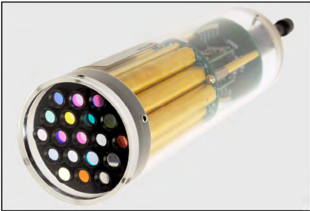
Fig. 30. A 19-channel radiance sensor built from microradiometers and using the architecture diagrammed in Fig. 27. The clear acrylic housing is for demonstration purposes only.
