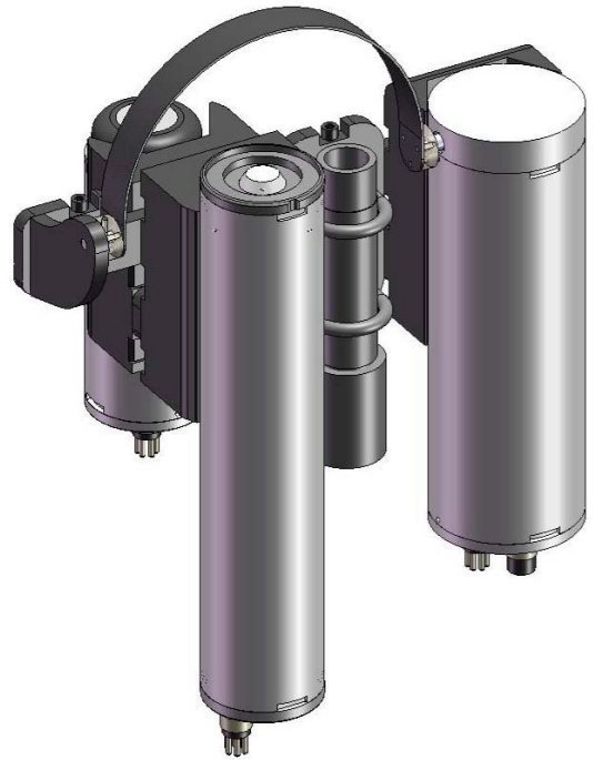
Fig. 50. A shadowband assembly schematic with a 19-channel microradiometer solar reference in the left foreground, the motor housing with supporting electronics at the right, and an optional BioGPS unit at the left rear. The narrow cylinder at center is the mounting post (1 in NPT 316SS pipe).
