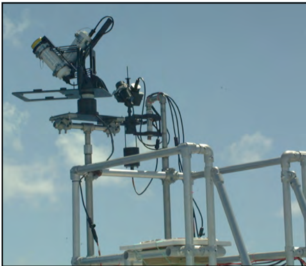
Fig. 8. The BioSORS (left) and microSAS (right) instruments mounted on the bow platform of the research vessel (R/V) Atalante during BIO SOPE.
