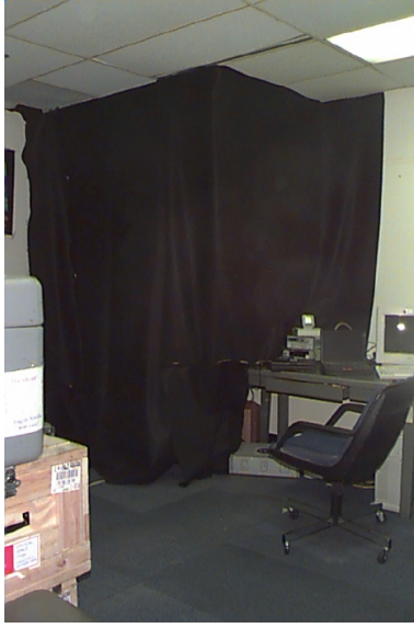
Figure 2.5: Pictures of the SIMBIOS optical laboratory. The left picture shows the curtains blocking the measurement area from ambient light, the right picture shows the measurement area.
