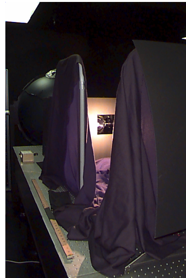
Figure 3.1: The picture on the left shows the setup for radiance calibrations with the FEL lamp at NRL, with a laser (at the left of the picture) for alignment purposes. The picture on the right shows the baffling for monochromator measurements of an FEL lamp at NRL.
