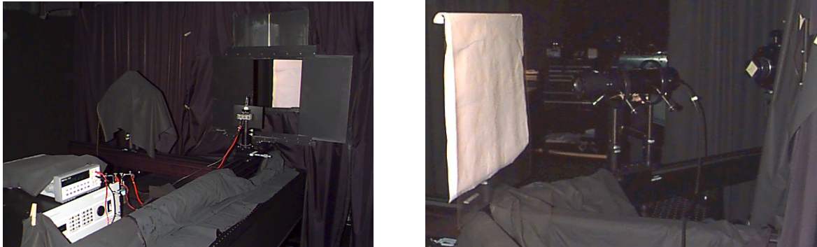
Figure 3.9: Left picture: Lamp holder on optical rail at Satlantic. The lamp power source can be seen on the left, the plaque can be seen through the square opening in the baffling wall on the right. Right picture: on the other side of the baffling wall, the Satlantic radiometer MVD046 (in the center) and SXR-II (on the right of the MVD046) measure the plaque (covered with a plastic sheet for dust protection in this picture).
